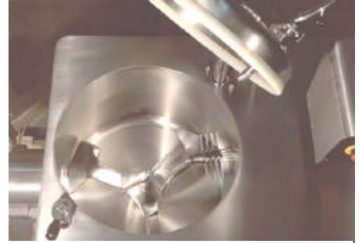
Stainless steel mixing bowl showing advanced-design impeller affixed to center-mounted vertical-shaft. Chopper is at right side.
